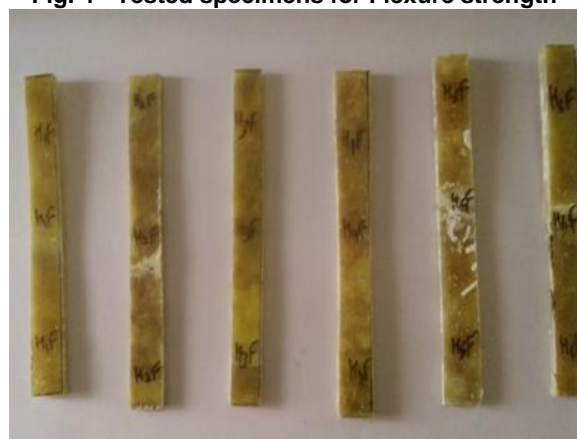
Fig. 4 - Tested specimens for Flexure strength
